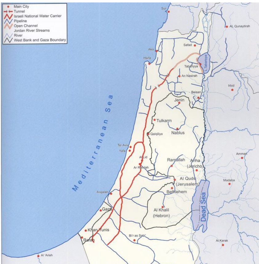
Main arteries of the NWC of Israel (in red), constructed between 1959 and 1964.
