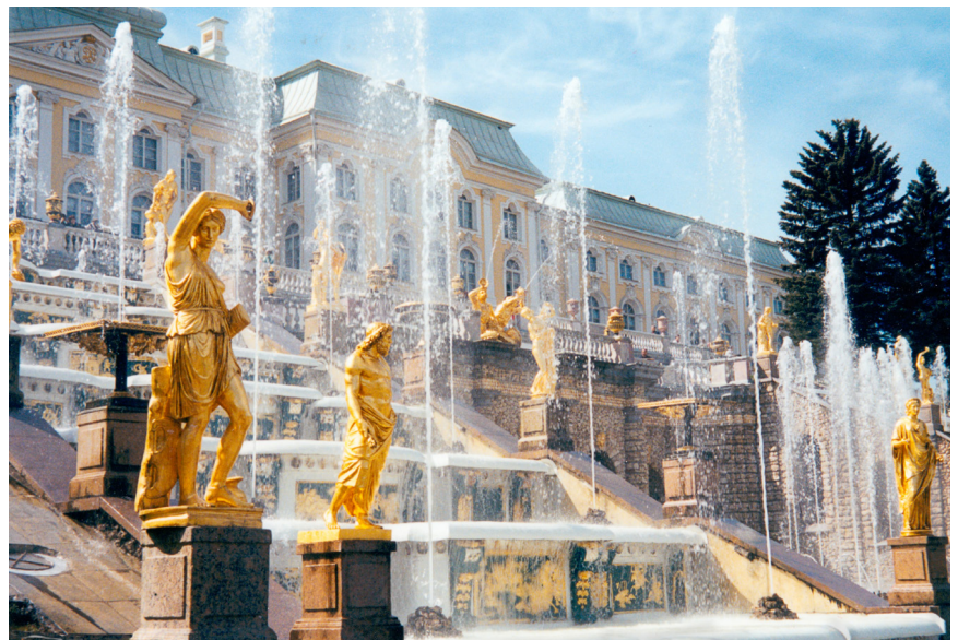
The Fountains of Peterhof Palace represent a technological advance where all the fountains operate without pumps. Water collects and is supplied from the Upper Garden's natural springs and reservoirs.
